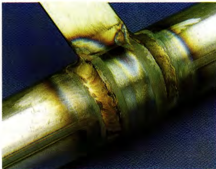
WELDED SAMPLE WITH DIL350
